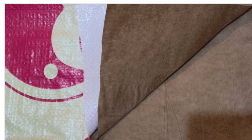
Printed woven PP valve bag with a kraft-paper inner ply
