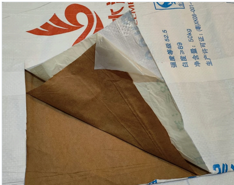
Cutaway: laminated woven PP outer, film and kraft-paper inner plies
